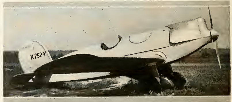
Cairns 90-horsepower model A monoplane with an all metal stressed skin
